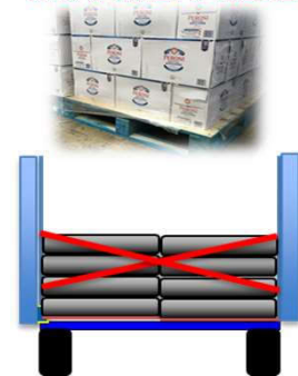
2 straps applied in a cross over rear pallets
