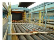
When 6m tubes loaded, all stanchions should be pulled in by ratchet straps Applied after second row of tubes
