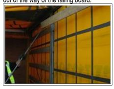
Stocksbridge Tata personnel have developed a prototype pole/'grabber' to assist with this operation and to try and eliminate the risk of Drivers being hit by the falling boards. We are looking to see if we can turn this into a workable solution.
