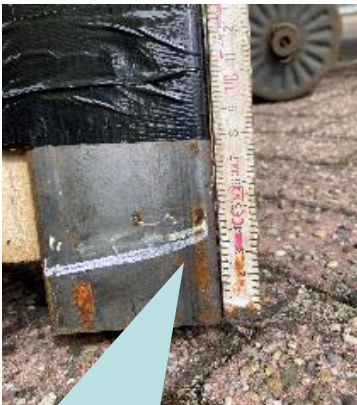
Chalk line shows 3cm max depth post was seated
